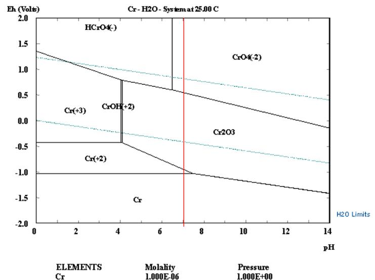
a.h. Nichro's hard chrome coatings do not contain any hexavalent chromium,  $\text{Cr}^{6+}$ . The coating consists of metallic chrome,  $\text{Cr}^0$ , which is neither dangerous to health nor to environment.
